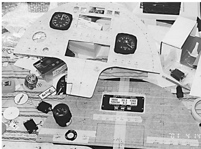
Laying out the real panel from the card board pattern
